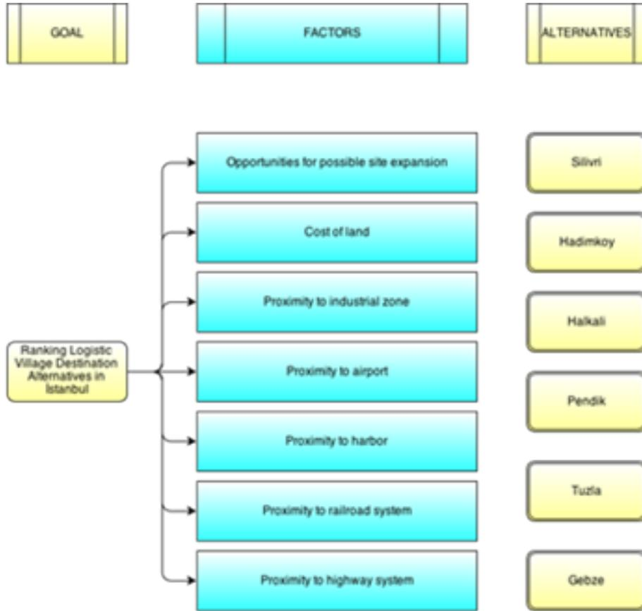
Figure 4. Hierarchical Structure for Logistic Village Evaluation
